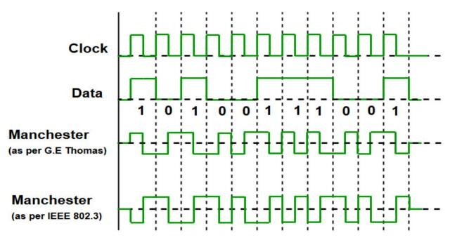
The binary data to be transmitted over the cable are not sent as NRZ [Non-return-to-zero].
